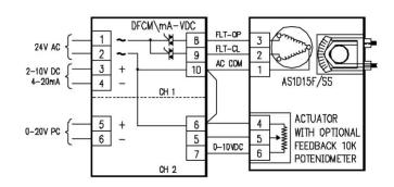
The DFCM/V-mA can be configured for feedback operation by inserting a jumper on J5. The channel 2 input Ai2 serves as the input for the feedback signal, a series resistor is used to bias the 10k Ohm potentiometer for a 0-10VDC.
